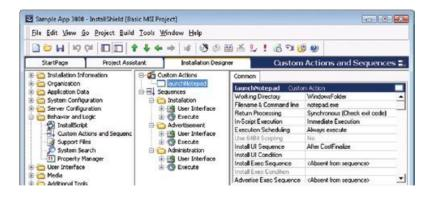
If the executable being launched is in a directory on the target system, the custom action must be placed after the standard CostFinalize action. The CostFinalize action sets the values of Directory properties, and an attempt to reference a Directory property (such as WindowsFolder or SystemFolder) will cause run-time error 2732, which is described in the Windows Installer Help Library as "Directory Manager not initialized".
